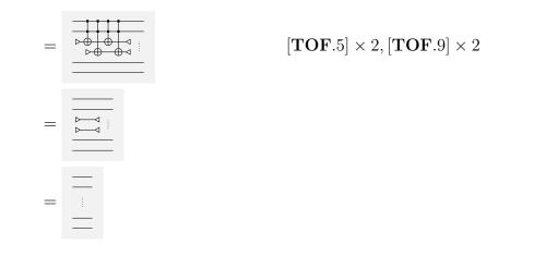
Next, we show how tof gates can be "pushed past" each other with a "trailing"  $cnot_n$  gate:
