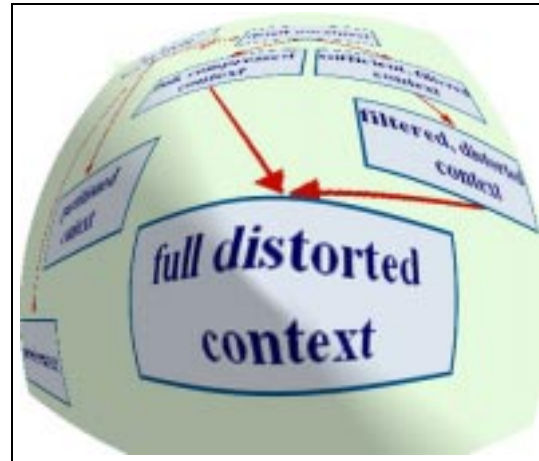
Figure 2.12: A diagram of a full distorted context. Note how the distortion continues right across the focus and note the extreme compression at the edges.
