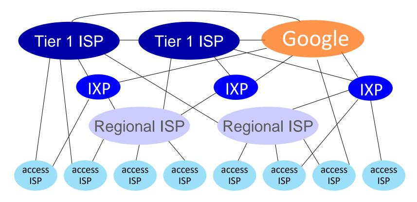
At "center": small # of well-connected large networks
