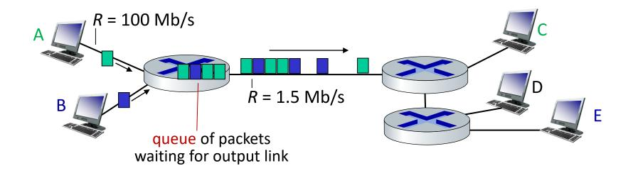
Packet queuing and loss: if arrival rate (in bps) to link exceeds transmission rate (bps) of link for a period of time:
