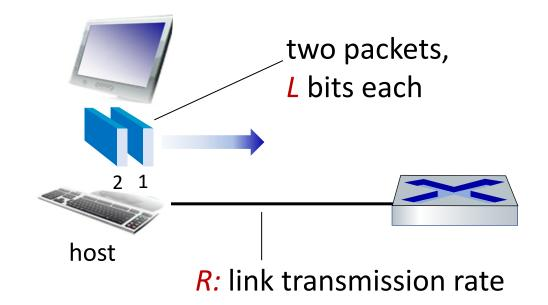
packet time needed to transmission = transmit
