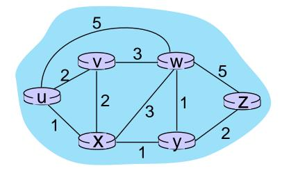
$c_{a,b}$ : cost of *direct* link connecting *a* and *b e.g.*,  $c_{w,z} = 5$ ,  $c_{u,z} = \infty$
