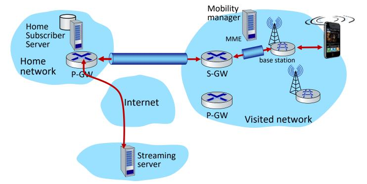
• tunneling via GTP (GPRS tunneling protocol): mobile's datagram to streaming server encapsulated using GTP inside UDP, inside datagram
