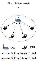
Fig. 5. An infrastructure WLAN consisting of an AP and N downloading STAs. The STAs communicate with servers in the Internet through the AP using long-lived Compound TCP connections. The servers are connected to the AP by high-speed wired links with negligible delay.
