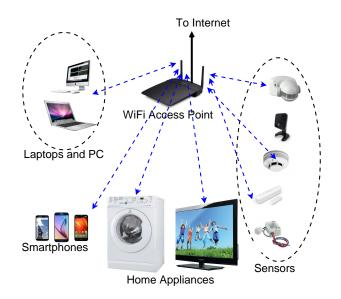
Fig. 1. IoT scenario consisting of sensors and devices, using Compound TCP over their WiFi interfaces. The WiFi Access Point (AP) is shared by all IoT devices.
