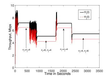
Fig. 18. Performance evaluation of buffer tuning algorithm when  $n_i$  and  $n_{j,(j\neq i)}$  changes over time using  $h_i^* = 0.526$  and  $p_w = 0.3$ .
