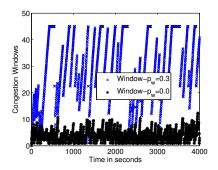
Fig. 12. TCP congestion window in packets when there are two SNR classes. SNR class 1 has error probability zero and class 2 has error probability 0.3.
