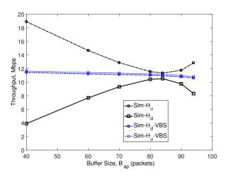
Fig. 17. Upload-download throughput unfairness with buffer overflows at the AP and fairness with VBS as observed in ns-2 simulations. There are five uploading and five downloading IoT devices both suffering from error probability  $p_w = 0.2$  and variable AP buffer.
