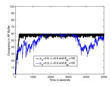
Fig. 14. AP buffer occupancy when there are two SNR classes. SNR class 1 has error probability zero and class 2 has error probability  $p_w$ . With the VBS algorithm, the occupancy  $\approx 60$  packets solves the starvation.
