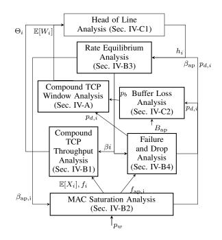
Fig. 6. Components and relationships in our Compound TCP model.
