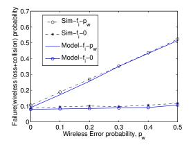
Fig. 9. Probability of transmission failure by the AP when there are two SNR classes. SNR class 1 has error probability zero and class 2 has error probability  $p_w$ .
