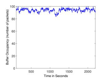
Fig. 2. AP buffer occupancy (in packets) with four Compound TCP connections. The AP buffer is almost always full.
