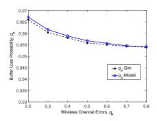
Fig. 13. Average buffer loss probability with increase in channel errors when there are two SNR classes. SNR class 1 has error probability zero and class 2 has error probability  $p_w$ .
