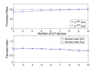
Fig. 8. Comparison of aggregate throughput and Jain fairness index in testbed experiments and simulations. Aggregate WiFi throughput increases with more IoT devices, but the fairness decreases.
