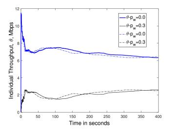
Fig. 3. Throughput unfairness between four Compound TCP connections over WiFi as observed in ns-2 simulations due to difference in wireless error probability  $p_w$ .
