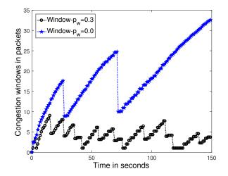
Fig. 4. Evolution of the TCP congestion windows with  $W_{\text{max}} = 45$ ,  $B_{\text{ap}} = 100$  packets and wireless error probability  $p_w$ .
