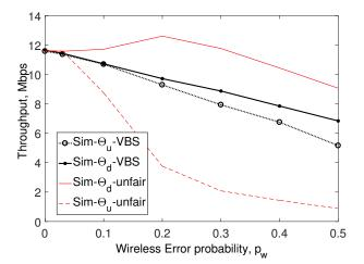
Fig. 16. Upload-download throughput unfairness with channel errors and fairness with VBS as observed in ns-2 simulations. There are five uploading and five downloading IoT devices both suffering from error probability  $p_w$  and large AP buffer.
