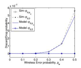
Fig. 10. Discard Probability at the MAC for the packets transmitted from the AP when there are two SNR classes. SNR class 1 has error probability zero and class 2 has error probability  $p_w$ .
