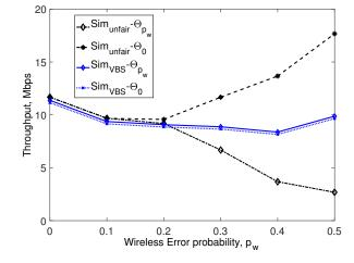
Fig. 15. Download-download throughput unfairness with difference in SNR and fairness with VBS as observed in ns-2 simulations. Class 1 has error probability 0 and class 2 has error probability  $p_w$  and there are five IoT devices in each class
