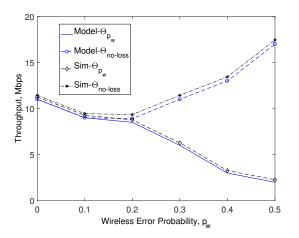
Fig. 11. Compound TCP Throughput obtained by each class when there are two SNR classes. SNR class 1 has error probability zero and class 2 has error probability  $p_w$ .
