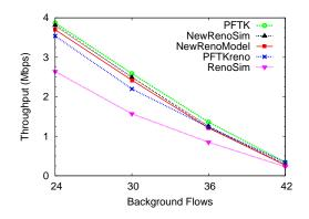
Fig. 11. Model Accuracy with Background UDP Traffic
