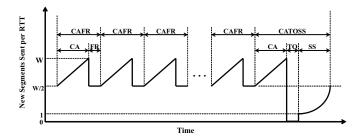
Fig. 5. Segment Transmissions in a Cycle (multiple CAFRs followed by CATOSS )
