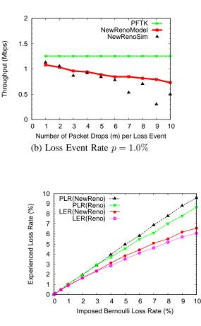
Fig. 8. Packet Loss Rate (PLR) and Loss Event Rate (LER) for the Imposed Bernoulli Loss Rate
