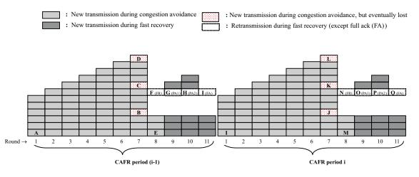
Fig. 2. Segment Transmissions in Two Adjacent and Identical CAFR Periods
