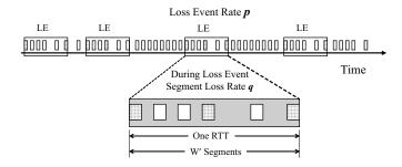
Fig. 1. The Two-Parameter Segment Loss Model
