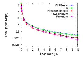
Fig. 7. Model Throughput Accuracy (log scale) with Bernoulli Packet Loss
