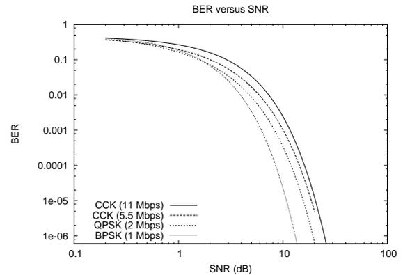
Figure 1. BER for IEEE 802.11b Modulation Schemes
