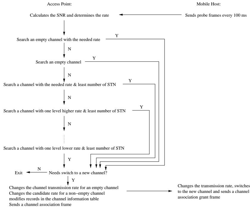
Figure 2. Flowchart of the Dynamic Rate Assignment Scheme
