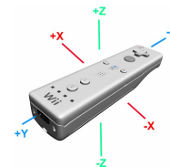
Figure 2. The coordinate system of Wiimote
