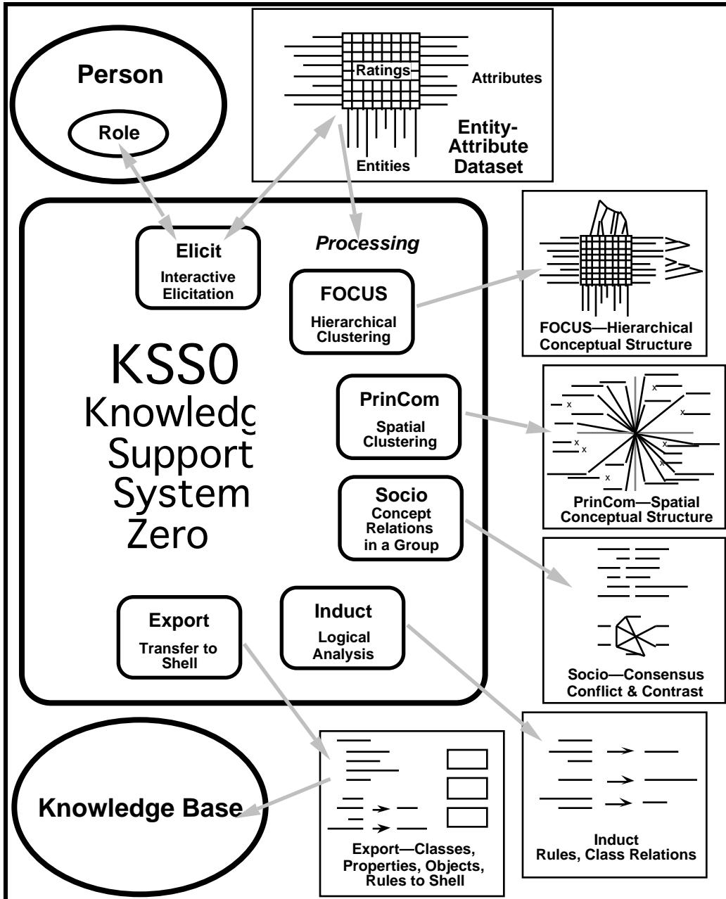
**Figure 3 KSS0, an integrated knowledge acquisition system**
