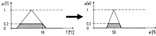
IF *temperature = medium* THEN *cooling valve = almost open*.
