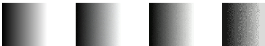
Figure 2.1: Illustration of 8, 6, 4, and 2 pixel bit depth, respectively
