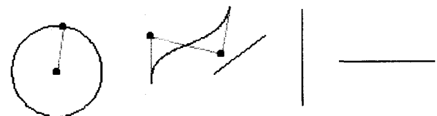
Figure 2 The program interprets the strokes as circle, cubic Bézier, line, horizontal and vertical lines
