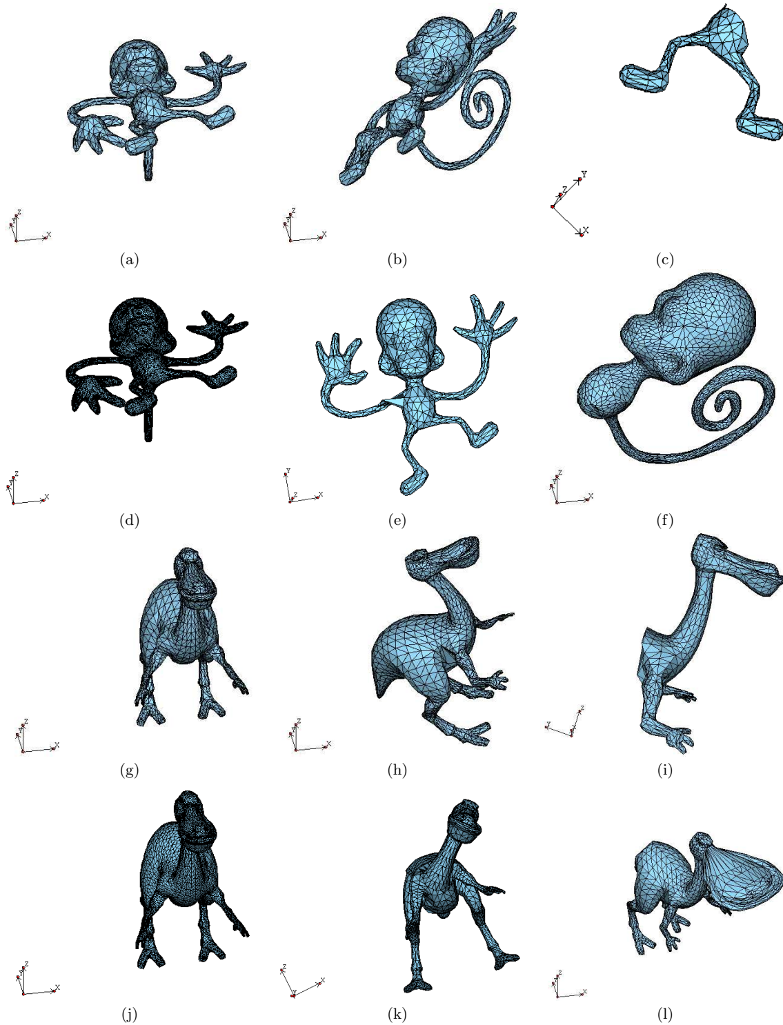
Figure 6: Watermarked monkey and dinosaur and effect of different attacks on them: (a) watermarked monkey (b) rotation (c) cut (d) subdivision (e) local rotation and translation (f) cut, subdivision, and rotation (g) watermarked dinosaur (h) rotation (i) cut (j) subdivision (k) local rotation (l) local scale, cut, change of format.
