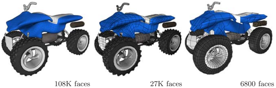
Fig. 13. Decomposition of a complex surface: with only 1/16th of the geometric detail, the rightmost surface is a faithful representation of the original
