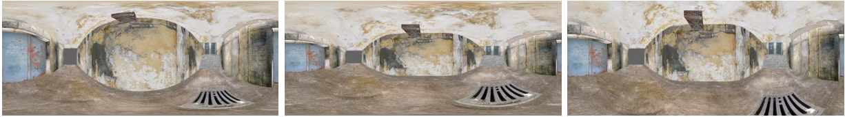
Fig. 15. Altering a spherical panorama (left) of a hallway to produce customized panoramic projections (middle and right).
