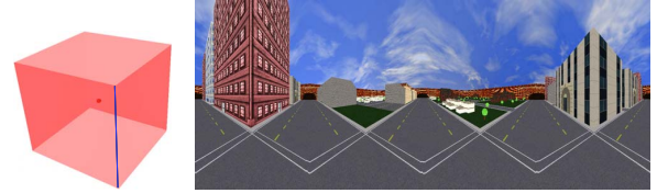
Fig. 5. A cubic panoramic projection surface with marked seam (left) and projected image (right).
