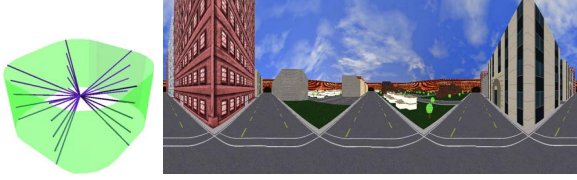
Fig. 12. A cubic panorama modified by smoothing the corners of the square outline. Resulting projection surface (left) and image (right). Compare with Figure 5.
