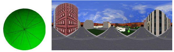
Fig. 4. A spherical panoramic projection surface (left) and projected image (right). The blue lines within the surface indicate rays that might be used to a column of the image.
