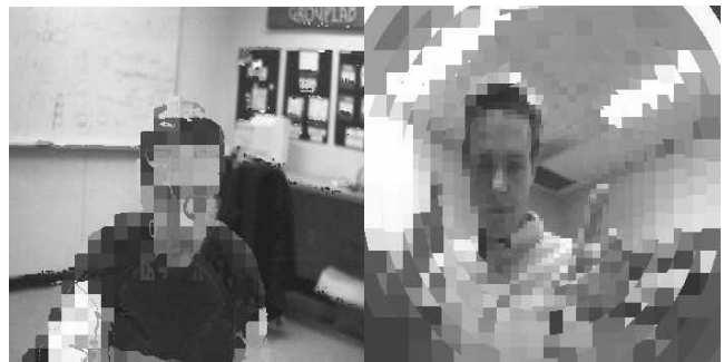
Figure 3. Pixelize filter used with two different excitory lenses: (left to right) activity selective, and radial.
