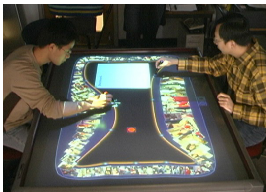
Figure 7.2: Example of two magnification areas on the peripheral Current, one for each participant.
