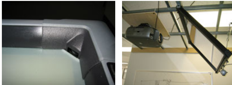
(a) Cameras in the corners of the SMART Board™. (b) Mirrors and projectors above the digital table.
