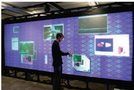
Figure 5. Interaction on a multi-projector large-scale wall display [6].
