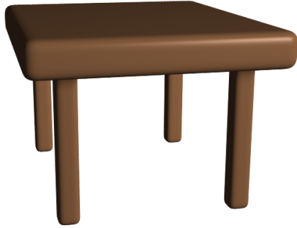
Figure 3: Five primitives with distance measured with L_4 blended to form a table.
