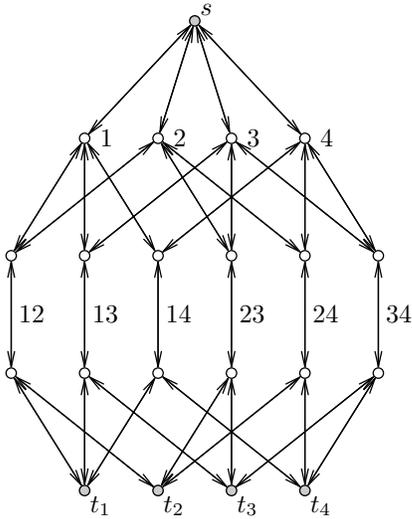
Fig. 4. The  $\alpha$ -balanced network  $ZK_\alpha(p=2, N=4)$ . Each downward link has capacity  $\alpha$ , each upward link has capacity 1.
