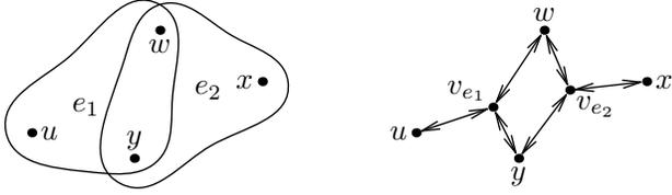
Fig. 5. A hyper-network (left) and its corresponding completely balanced bipartite network (right).
