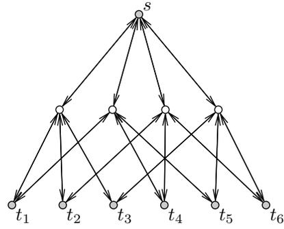
Fig. 3. The  $\alpha$ -balanced network  $C_\alpha(n = 4, k = 2)$ . Each downward link has capacity  $\alpha$ , each upward link has capacity 1.
