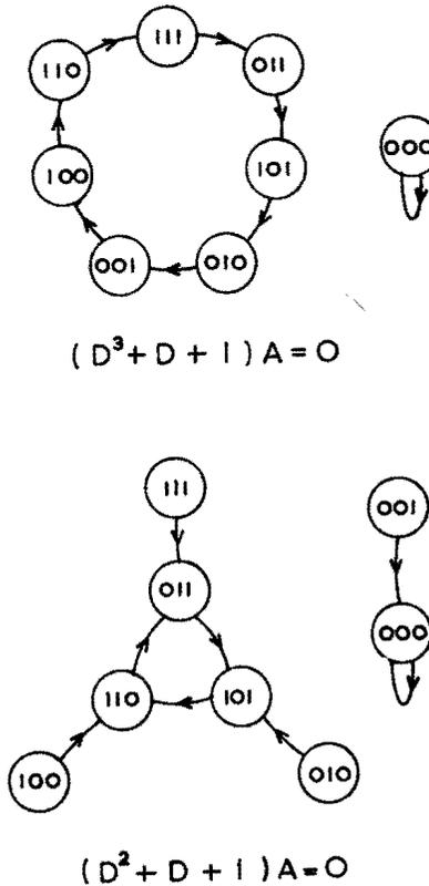
Fig. 27. State trajectories for feedback shift registers.
