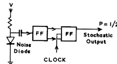
Fig. 25. System for generating output of probability  $\frac{1}{2}$ .
