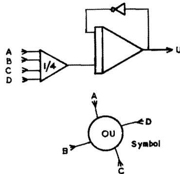
Fig. 35. "Laplacian" element.
