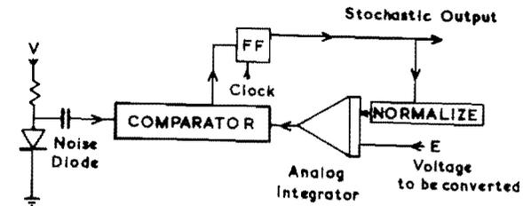
Fig. 23. Analog-to-stochastic converter.
