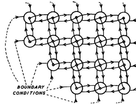
Fig. 36. Network of "Laplacians" for solving Laplace's equation.
