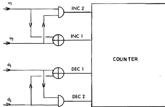
Fig. 11. Two-input summing integrator for representation II.
