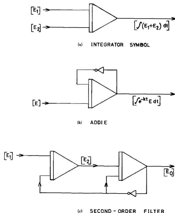
Fig. 14. Integrator configurations.
